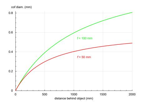
The slopes of both graphs are virtually identical out to well beyond where the diameter of the circle of confusion is 0.03 mm, showing that to a first approximation both lenses have the same depth of field. However, the size of the circle of confusion for in infinitely distant point is twice as large for the 100 mm lens (1.25 mm) as for the 50 mm lens (0.625 mm).
